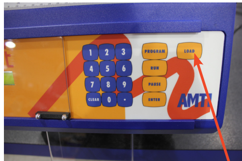
8. HIT "LOAD" KEY AND SLIDE KEYPAD SAFETY SHIELD BACK TO RIGHT.
