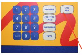
11. TO STOP CONVEYOR: PRESS "RUN/STOP" BUTTON AND CONVEYOR WILL STOP.
