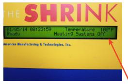
3. LCD READOUT SHOWING HEATING SYSTEMS OFF.
