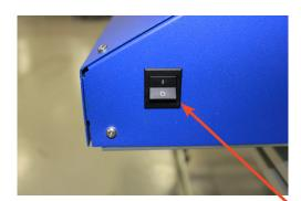
NOTE: SHRINK OVEN WILL AUTOMATICALLY SHUT DOWN IN APPROXIMATELY 5 MINUTES OR YOU CAN PRESS THE "ON/OFF" SWITCH TO OFF WHEN TEMP SHOWS 200 DEGREES.
