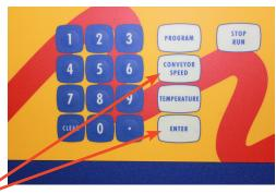
6. CONVEYOR SPEED: PRESS "CONVEYOR SPEED" BUTTON, KEY IN DESIRED SPEED, THEN PRESS "ENTER".
