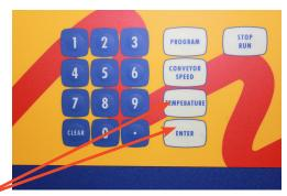
4. TEMP: PRESS "TEMP" BUTTON AND KEY IN DESIRED TEMP, THEN PRESS "ENTER" BUTTON.
