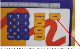
5. TO LOAD MATERIAL, PRESS "LOAD" BUTTON. - MATERIAL WILL INDEX AND COMPLETE ONE CUT CYCLE.
