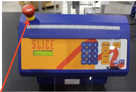
Emergency Stop Button
